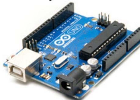
Fig. 3. Arduino Uno Board [16].
