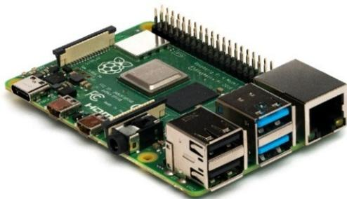
**Fig. 8.** Raspberry Pi Board [23, 24].
