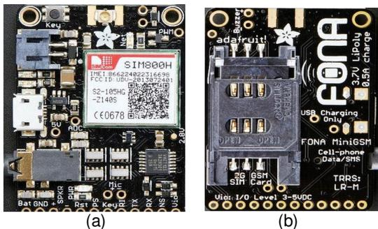
Fig. 18. Adafruit FONA module (a) front view and (b) back view [36, 37].
