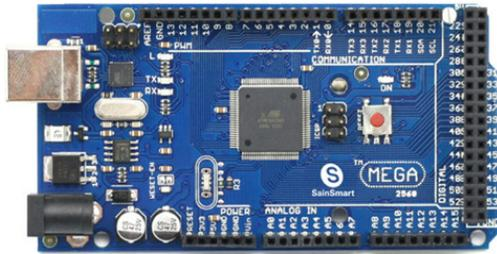
Fig. 5. Arduino Mega2560 Board [19].
